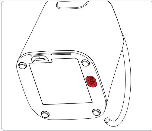
3. Turn on the Power switch located on the underside of the unit. A Green LED will flash on the top of the unit for 30 seconds.
