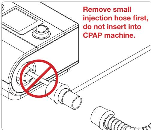
**Without humidifier:** If you are not using a humidifier, remove the short length of black hose from the inside of the injection fitting by pulling it straight off, and then attach the fitting directly to your CPAP machine. Reconnect your CPAP hose to the end of the injection fitting.
