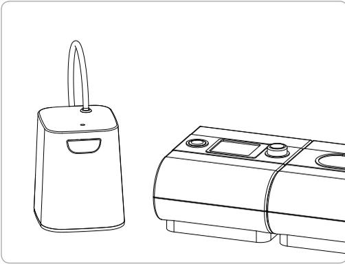
The SoClean 2 Go sanitizes by pumping activated oxygen into your humidifier reservoir and through your CPAP hose. It then passes through your mask into the mask bag, where it sanitizes your mask inside and out. Finally, it exits the mask bag by passing through a filter that converts it into ordinary oxygen.
